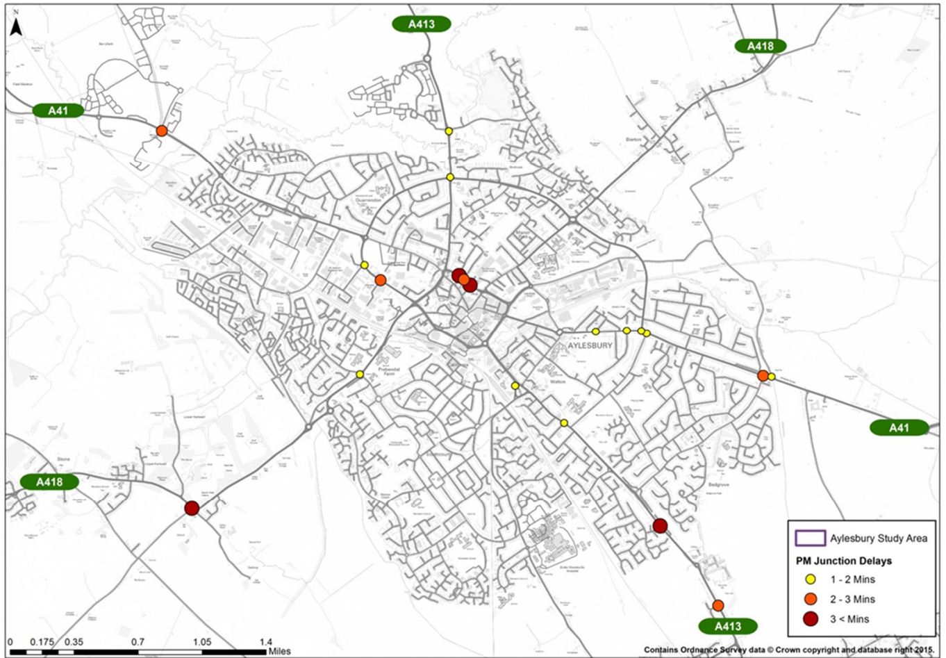
Figure 3.18 – PM Peak Junction Delays in Aylesbury
